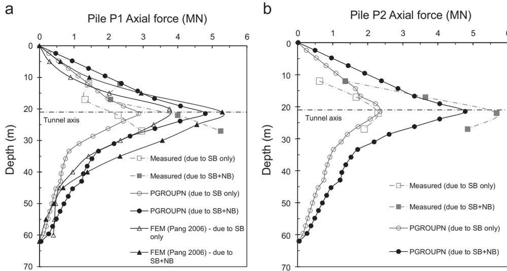
Fig. 19. Measured and computed axial force distributions for (a) pile P1 and (b) pile P2.
