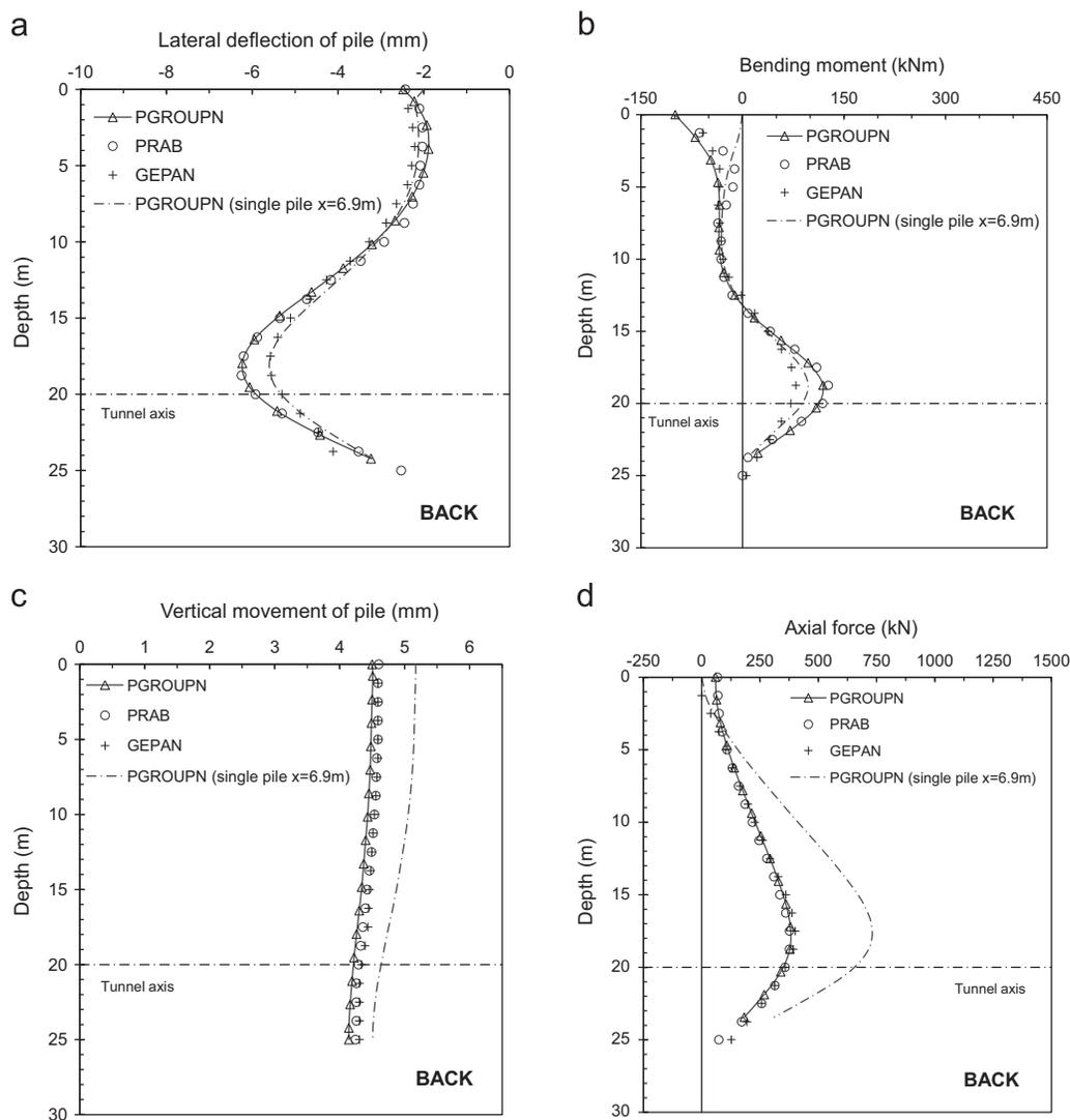
Fig. 6. Comparison of pile-group responses for back pile.
