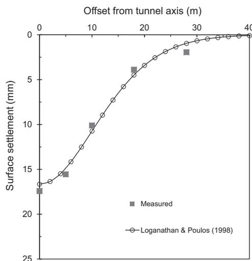
Fig. 12. Measured and computed free-field surface settlements.
