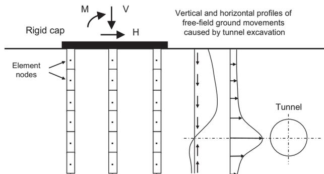
Fig. 1. BEM schematisation of the problem.
