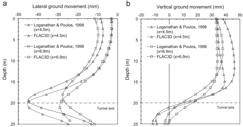
Fig. 7. Comparison of computed free-field ground movements.
